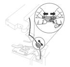
3 Rotate the hinge lever counterclockwise. Lift the top hinge free of the hinge lever latch.
