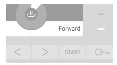
Press button Open the door (is not lit!). The programme will be interrupted and the door unlocked.
