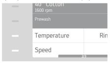
Tapping the light bar next to **Speed** reduces the spin speed in steps of 100 rpm
