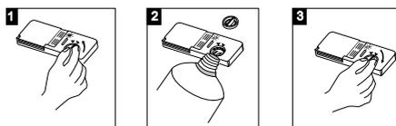
1. To open the dispenser, turn the cap to the "open" (left) arrow and lift it out.
