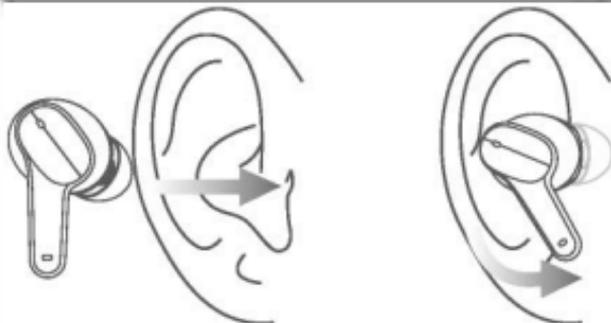
Put the earbuds in your ears, rotate and adjust it to the best angle. Be sure to wear comfortably and secure fit.
