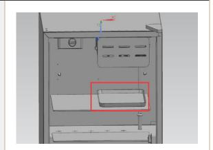
2) Replace the drain tray, the reverse process can complete installation, And place in the graphical position.
