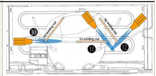
12) Replace the filter, Cu-Fe tubes welding 13 used Ag welding rod, Cu-Cu tubes welding 14 used Cu welding rod.
