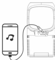
1) Plug Aux cable in the «AUX» jack, another end inserts to the computer or other audio device, it automatically enter AUX in mode or short press **⏻** to enter Aux in Mode from bluetooth
